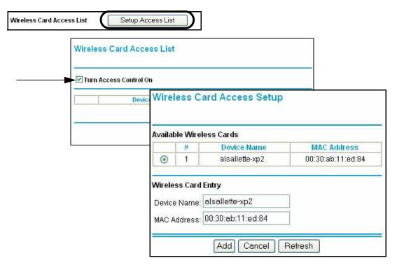
Figure 4-5: Wireless Card Access List Setup
